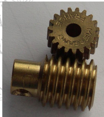
Figure 7: inside the motor gear of two worm wheels
